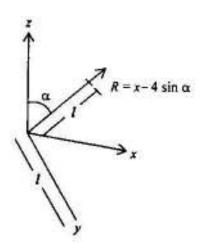
A V-shaped antenna is shown in the above figure. The current distribution on the antenna is given by  $I = I_0 \cos(K_0 u)$  and the length of the antenna is l. Find the maximum field strength along the x-axis if  $l = \frac{\lambda}{4}$  and  $\alpha = 45^{\circ}$ .
