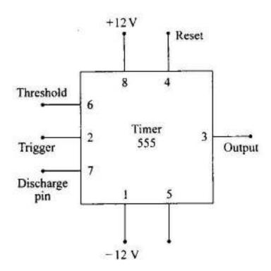
In the IC Timer 555 shown in the above figure determine the reference levels for the two comparators inside the chip. Justify your answer by drawing a block diagram of the internal circuit of IC Timer 555.
