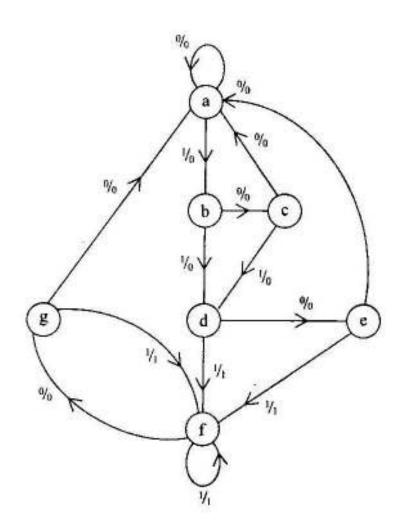
There are infinite number of input sequences that can be considered. Consider the input sequence 01010110100 starting from the initial state 'a'.
