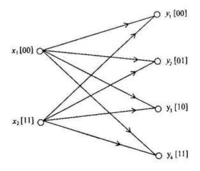
Calculate the rate of joint information transmission for the above channel. Assume  $p(x_1) = p(x_2) = \frac{1}{2}$  where  $[X] = \{x_1, x_2\}$  is the set of input symbols.
