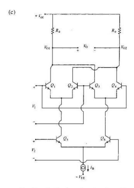
For the circuit shown in the above figure determine by relevant analysis, under what conditions the output voltage is proportional to the multiplication of the two inputs  $V_1$  and  $V_2$ . Derive an expression for  $V_0$  in terms of  $I_B$ ,  $V_1$  and  $V_2$ .
