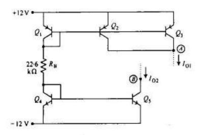
Assuming matched transistors with large  $\beta$  (i.e. negligible base currents), determine the currents  $I_{01}$  and  $I_{02}$  in the circuit given in the above figure. Assume that nodes B and A are connected at appropriate voltages which ensure that transistors  $Q_5$ ,  $Q_2$  and  $Q_3$  are in active region.
