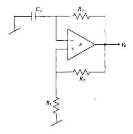
Assuming the gain A of the op-amp to be represented by  $A \cong \frac{\omega_I}{s}$  where  $\omega_I$  is the gain-bandwidth-product of the op-amp, analyze the given circuit and determine under what condition, the circuit can generate sinusoidal signal at the output? What is the frequency of the output waveform if  $R_1 = 1 \ K\Omega$ ,  $R_2 = 9 \ K\Omega$ ,  $C_0 = 0.1 \ \mu F$  and  $R_0 = 10 \ K\Omega$ ?
