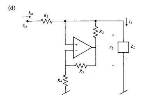
Explain the operation of the circuit shown in the above figure and determine under what condition the output current  $(I_L)$  can be made independent of load voltage?
